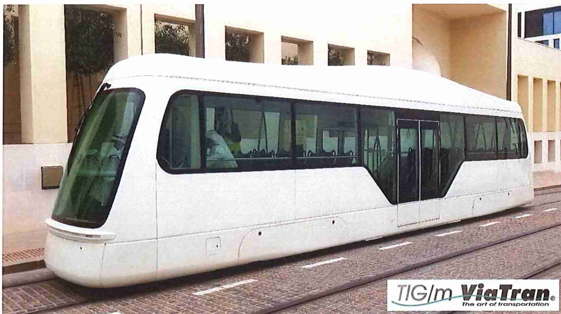
Figure 1-6, TIG/m MRV-3AC 100 passenger Modern Tram:
