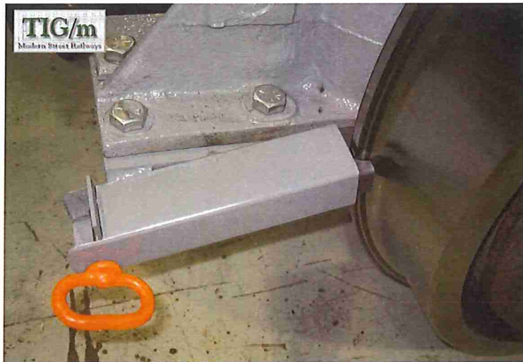
Figure 1-5, TIG/m proprietary flange lubrication system:
