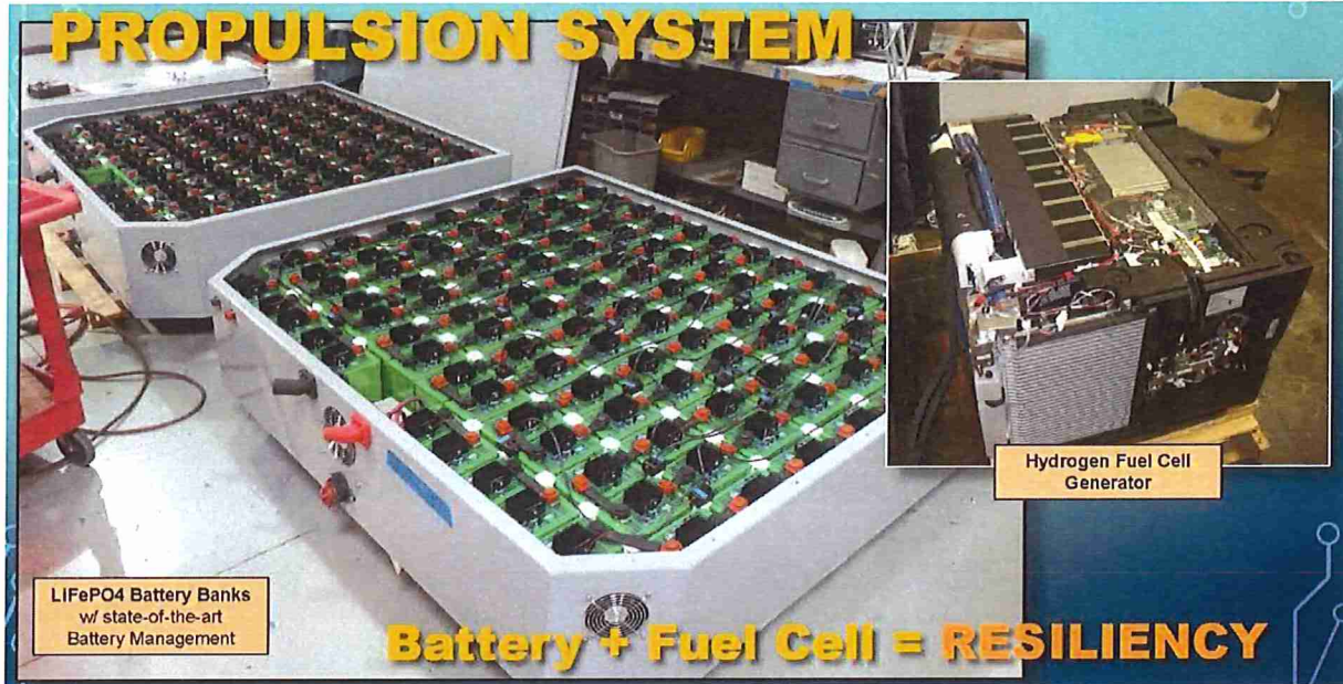
Figure 1-3, Battery Dominant Propulsion system:
