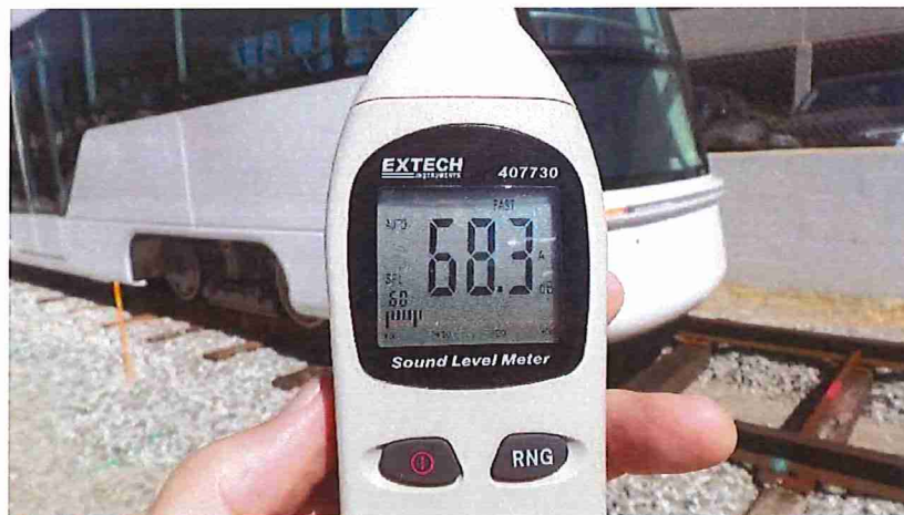
Figure 1-4, dB rating of operational TIG/m Tram:
