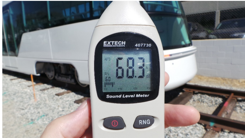
Figure 1-4, dB rating of operational TIG/m Tram:
