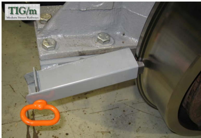
Figure 1-5, TIG/m proprietary flange lubrication system:
