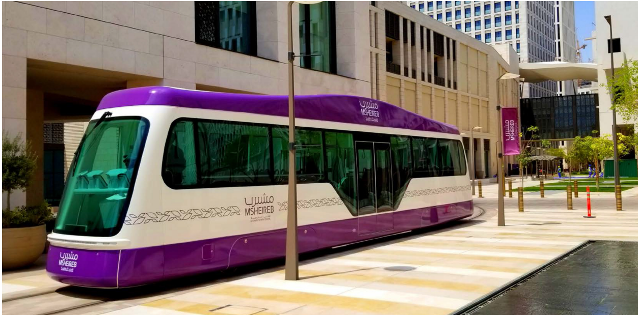
Figure 1: MODERN STREETCAR - TIG/m MRV-3AC single body (passenger capacity 100)
