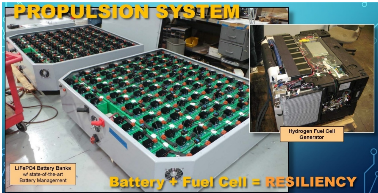
Figure 1-3, Battery Dominant Propulsion system:
