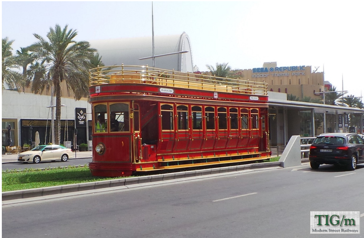
Figure 1-11, TIG/m Convertible Double-Deck Trolley in closed configuration for summer in Dubai.
